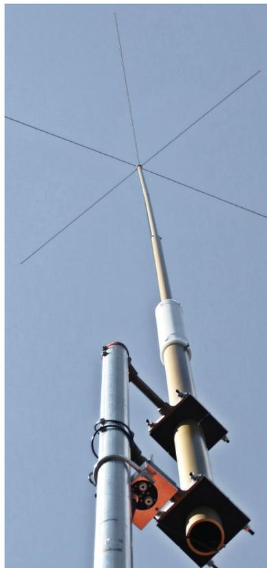
band due to the longer wavelengths, but despite its small stature, the HPR.0990 can still produce efficiency of 55 mV/m per kilowatt at 540 kHz.
